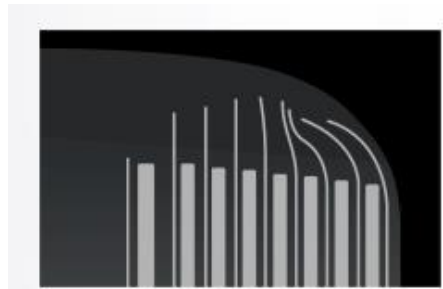
The negative electrode was deflected in the upper-right corner of the battery
