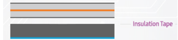
A number of batteries were missing insulation tape
